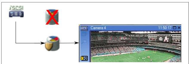
When the Secondary VRM and the optional Secondary Failover VRM are both not connected, the encoder provides playback. Close the Image pane and drag the camera again to an Image pane:
