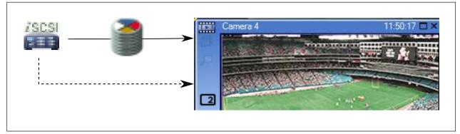
When the Secondary VRM is not connected, the configured Failover VRM provides playback. Close the Image pane and display the camera again in an Image pane:
