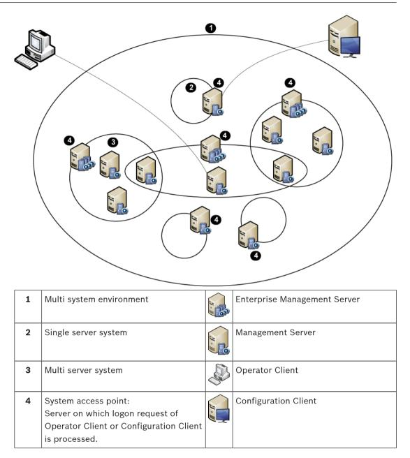
When a client logs on to Enterprise Management Server, it is possible to get access to all Management Servers of this Enterprise System simultaneously.
