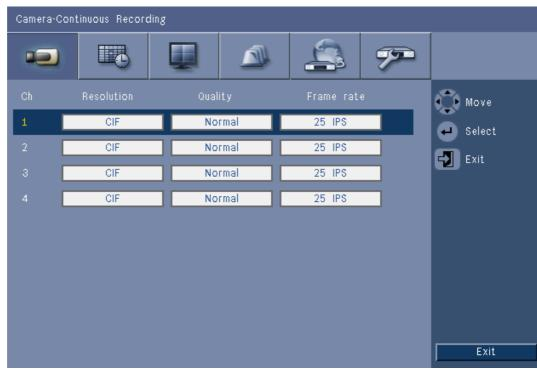
**Figure 6.5** Camera - Continuous Recording Continuous recording mode:
