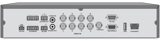
Figure 3.1 Back panel connections for the 4-channel model\*
